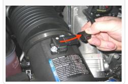
3. Loosen both hose clamps and remove the OE intake tube from the vehicle.
