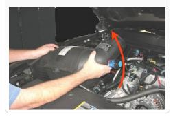
5. Make sure that the OE grommets are still in place in the OE air box tray. They may have pulled out with the air box removal.
