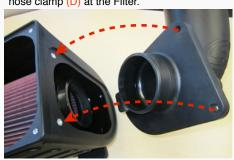
8. Remove the OE Filter Minder and OE Grommet. Insert the grommet into the Filter Adapter Tube (B). Then push the Filter Minder into the grommet.
