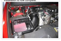
11. Test fit the Air box assembly. If there is a clearance issue with the Air Box (A) it may be necessary to loosen the bolt at the base of the coolant overflow/ reservoir then slide the reservoir back and retighten the bolt.
