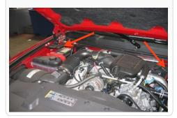
2. Disconnect the electrical connection at the MAF sensor on the OE air box tube.
