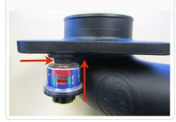
9. Remove the MAF sensor from the OE air box using the supplied T-20 Torx wrench. Make sure the rubber seal stays with the MAF sensor.
