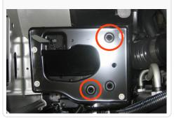
6. Remove the headlight housing bolt in the radiator core support between the passenger side fender and the hood bumper.
