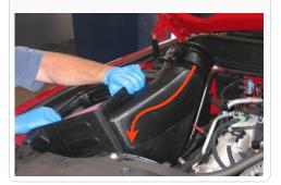
15. With a #64 Hose Clamp (E) and a #72 Hose Clamp (F) installed on the Straight Coupler (N), secure the smaller end to the Intake tube (L).
