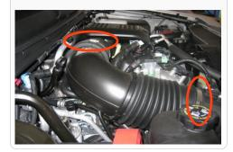
4. Pull up on the OE air box to remove it from the vehicle, there are two press prongs that go into rubber grommets on the bottom side.
